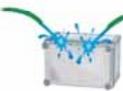
防护从每个方向对准箱体的低压喷水<br>protected against low pressure jets of water from all directions-limited ingress permitted | 09    |
