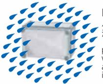
防护以60°角从垂直线两侧溅出的水<br>protected against water sprayed from all directions-limited ingress permitted              | 07    |
