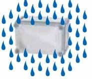
防护垂直落下的水滴<br>protected against vertically falling drops of water                                                 | 01-05 |
